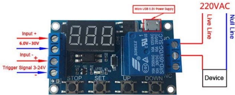
Low Voltage Control High Voltage Connection Picture
